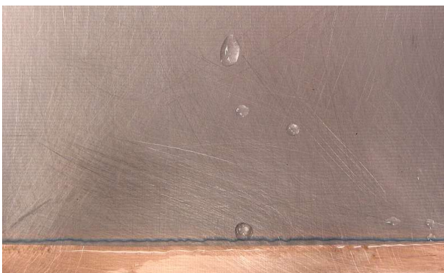
Illustration 1: Successful wet lamination of dry film on blank PCB material
