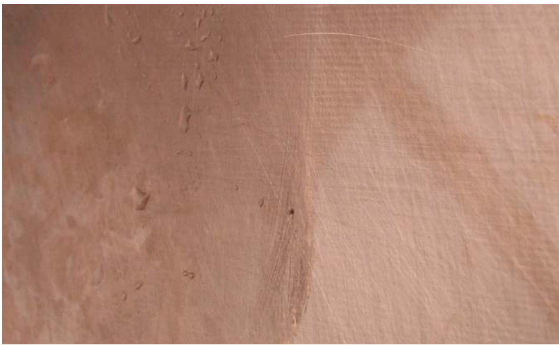
Illustration 2: Showing both a contaminated (left side) and clean (right side) surface. Note the water beading on the contaminated side.
