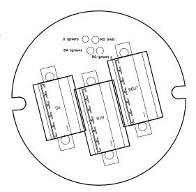
LED RD (red) Following IBS-Interface is disconnected
