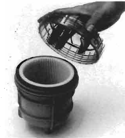
Controle koelwaterfilter. Checking raw water strainer.
