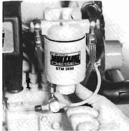
Waterafscheider aftappen. Draining water separator.
