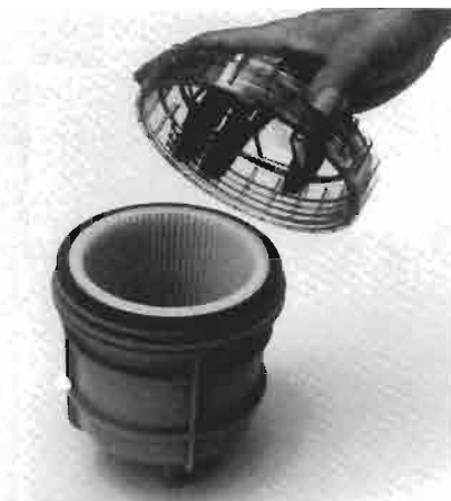
Controle koelwaterfilter. Checking the raw water strainer.
